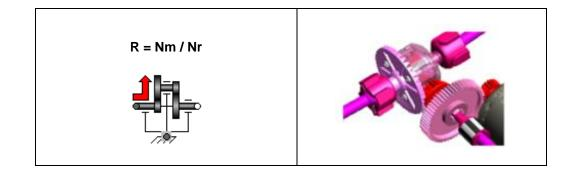
It is the product of two reductions: The first with the gear and the cogwheel at the engine's output, The second is at the differentials' gears.
