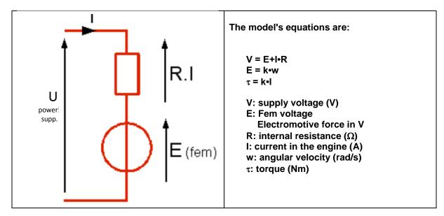
Internal resistance of the engine:
