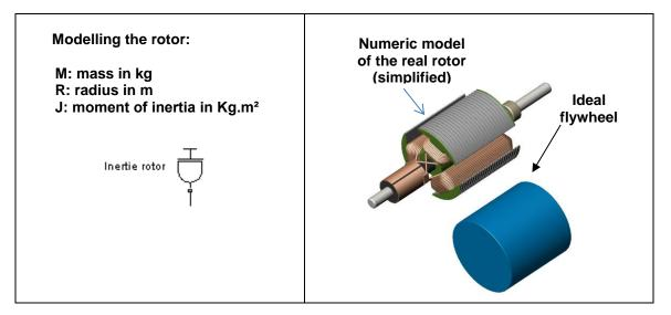
It would be easy to calculate the moment of inertia of the rotor if it were cylindrical and made of solid steel with a density of 7800kg/m<sup>3</sup>. The flywheel includes hollow and solid parts, but we can model it as a cylindrical flywheel with the same dimensions but with a lower average density of 3000kg/m<sup>3</sup>.
