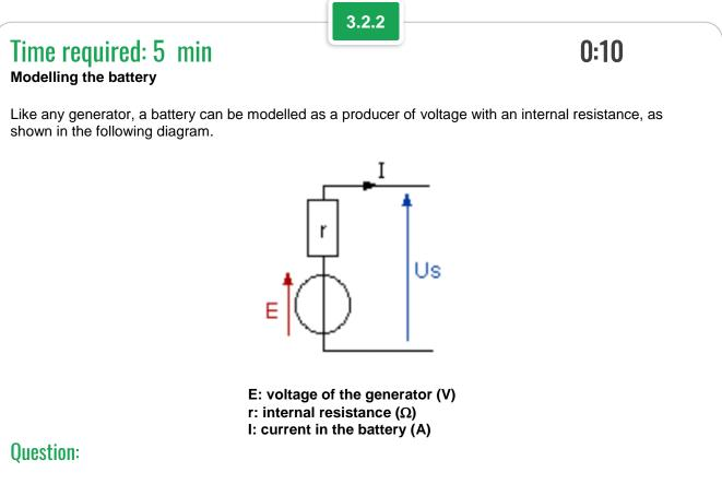
Measure the voltage on a charged battery and complete the command circuit model of the generator using that voltage.
