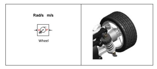
As in both cases, the denominator is in seconds, we have to determine the ratio between the wheel's angle of rotation in radian and the distance travelled by the wheel in meters (see page 12).
