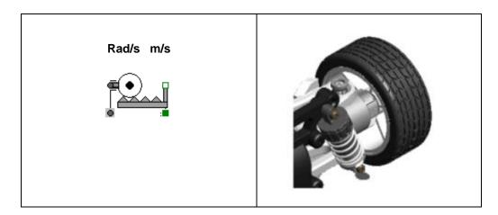
As in both cases, the denominator is in seconds, we have to determine the ratio between the wheel's angle of rotation in radian and the distance travelled by the wheel in meters (see page 12).
