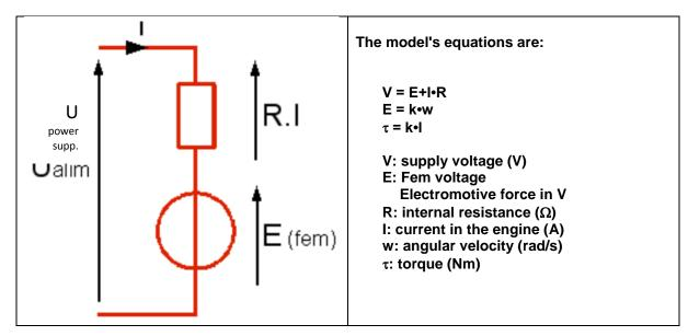
Internal resistance of the engine:
