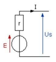
E: voltage of the generator (V) r: internal resistance ( $\Omega$ ) I: current in the battery (A)
