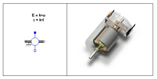
Measuring torque is tricky, so we will measure speed in order to determine the value of the coefficient.
