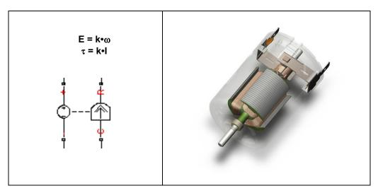
Measuring torque is tricky, so we will measure speed in order to determine the value of the coefficient.
