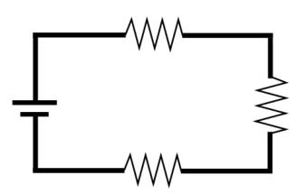
Fig. 1 Series circuit (with 3 resistors)
