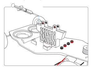
Step 2. Take the metal made anode and clips it into the cathode as show below
