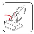
Notes: Once the fan stops rotating, open the clamp to purge some solution out of the fuel cell and close the clamp. Wait for 5-10 minutes, the fan should start rotating by itself once connected. If the fan does not run at this time, it may need to be flicked with your finger to start.
