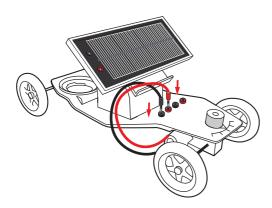
Step 4. Connect the solar panel and the car using the two remaining wires. Ensure to respect the polarity shown by the color code.
