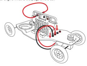
Step 4. Connect the black long wire in the central plug and the red on in the front red plug. Connect the other end of these wires into the car right plugs. The car starts to move. Ensure that you have connected the wires in the good sense. On the contrary, the car will go back.
