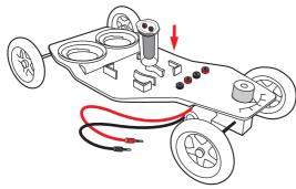
Step 2. Connect the engine wires which exceed the bottom of the car, to the closest red and black plugs.
