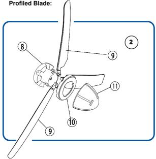
Place the Rotor Base (8) onto the flat surface of a table. Install 3 pcs of the same type of profiled blades (marked B or C) evenly on the Rotor Base. Pay attention that the snap joint must be pushed into the Rotor Base. Place the Blade Holder (10) on top of the installed blades. Pay attention to the direction of the Blade Holder. Screw the Blade Assembly Lock (11) onto the top of the Blade Assembly.
