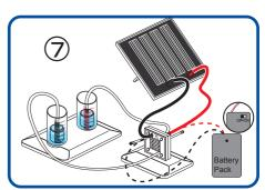
As sson as the electrolysis is completed, you can use the energy contained in the hydrogen tank to power other systems. Please refer to the experiment 3-6 in Wind Energy chapter.
