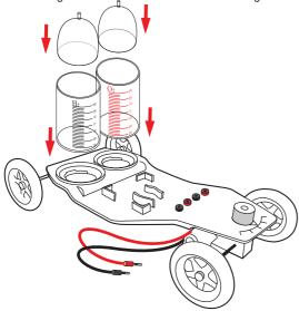
Step 5. Fill the containers with 40ml distilled water.
