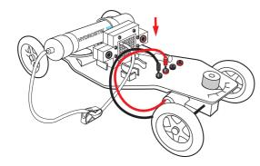
Step 7. Connect the two wires to the red and black plugs on the car frame. Connect the other end to the fuel cell.
