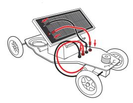
Step 5. Place the car under direct strong sunbeams to make it run.
