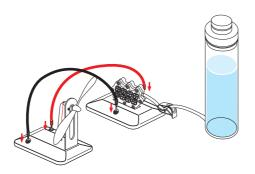
**Step 7:** Open the clamp. You can notice the liquid flows out of the tube through the fuel cell. Once you see the liquid flows out of the tube, close the clamp.
