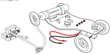
Step 6. After this place the mini fuel cell on the slot located on the car frame top. Ensure they fit well. Then connect the car engine wires into its plugs.
