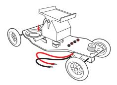
Step 2. Place the solar panel as shown in the picture below. Remind that the plugs have to be on the right side when you face the car.
