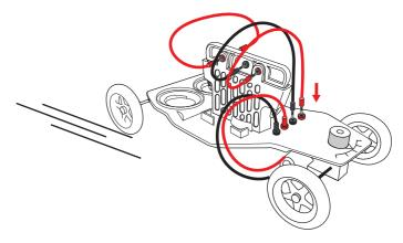
Note: After long time running, the car speed will slow or stop. If you want to continue to run the car, you should pull out the anode metal plate to clean it up with the running water. Replenish some salt solution to the fuel cell tank. Place back the anode metal plate to the cathode fuel cell tank, the car will continue to run. After use, you should pull out the anode metal plate and clean up the fuel cell tank with the running water. Keep them dry for storage.
