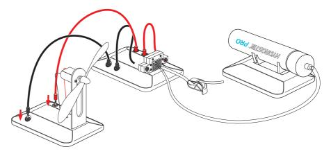
Now you may use a multi-meter (not provided) or Horizon's REM to measure the output voltage & current produced by the fuel cell or do various experiments.
