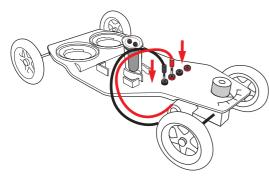
Step 3. Connect the capacitor and the car using the two remaining wires. Ensure to respect the polarity shown by the color code. The car will start to move immediately. If you connect wires in the wrong sense, the car will go back.
