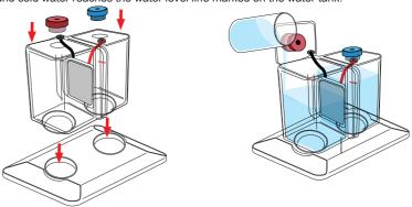
**d.** Insert the thermometers in the holes of the seals carefully and slowly until it almost reaches the bottom of the tank.
